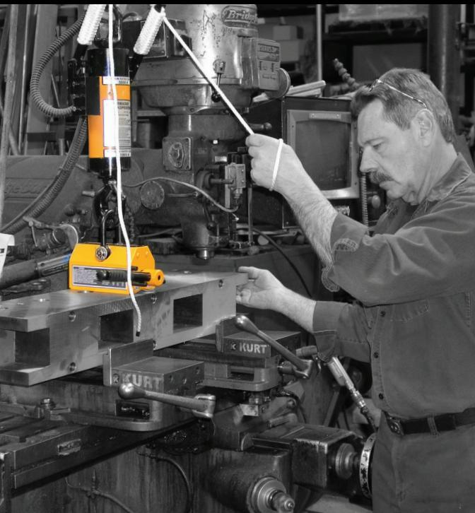
**Permadur Vacuum Lifting Systems** provide safe, efficient handling of non-ferrous and delicate materials. Designed for glass, steel, aluminum, composites, sheet goods, they feature custom pad arrangements to suit unique requirements. Powered by electric, air, or battery, these systems reduce operator strain while preventing surface damage.
