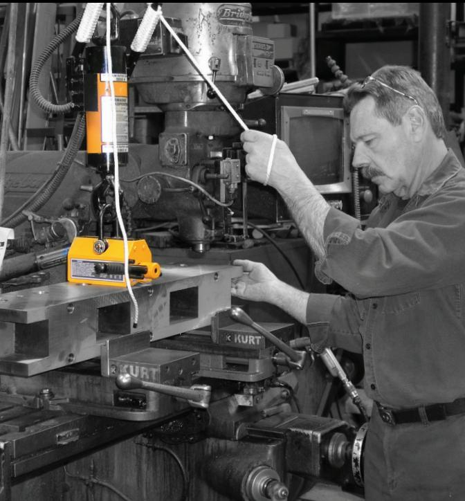
**Permadur Plate Handling Systems** are engineered for safe, efficient movement plate steel. Built with fail-safe magnet technology, they prevent accidental load drops, even during power failure or misoperation magnet control. Available in AC or battery-powered options, they are tailored for plate size, thickness, and handling requirements.
