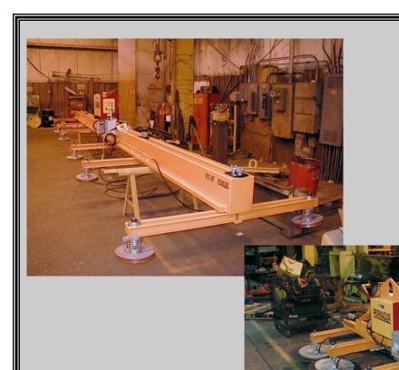
The above pictured Systems are a *PERMADUR* Series 612 and Series 408 Plate Handling Systems. These Systems consisted of a 1500 and 750 Power Pac respectively. These Systems were built for one Customer and were set up so that they could be Suspended from the same Crane and the Controls were set up to support an interface with ON/OFF/OFF controls on the Hoist Pendant/ Crane Radio Controls.
