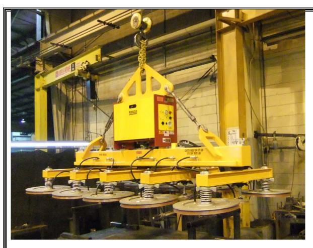
The above pictured System is a *PERMADUR* Series 515 Plate/Part Handling System. This System consisted of a 1500 Power Pac and fifteen Vacuum Pads on a 10' Load Beam. Ten VPN-20-30 Vacuum Pads and 5ea. VPN-6SO-30 Pads on five Crossarms support 8'x 12' Plate Loading (up to 4" Thick). The System Load beam was designed to be attached to a Single Hook Crane via the bail and Turnbuckle Sling on the Power Pac. The System is powered by a 460 VAC power supply.
