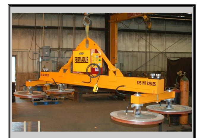
The above pictured System is a **PERMADUR** Series 204Plate Handling System. This System consisted of a 330 Power Pac with a Structural Sling, two 3' **Crossarms, and four Vacuum** Pads on a 10' Load Beam. The four VPN-24-30 Vacuum Pads support the loading of 6'x20' Plate, 1/4" - 1-1/2" Thick, 8000# Max Load. The System Power Pac which utilizes a 115 VAC **Power Supply includes Remote ON/OFF** pushbutton Control Pendant and Safety Indicator Lights.
