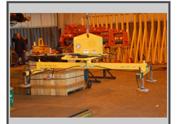
The above pictured Vacuum Lifting System is a PERMADUR Series 204 Plate Handling System. This System consisted of a 250 Power Pac and four Vacuum Pads on an 8' Load Beam. The four VPN-6SO-30 Vacuum Pads are positioned on 2ea. 3' Crossarms. The Controls consist of an ON/OFF Slide Valve mounted on an operator guide handle that is adjustable up to 30" from Power Pac. Power Pac utilizes 115 VAC Power Supply by customer.
