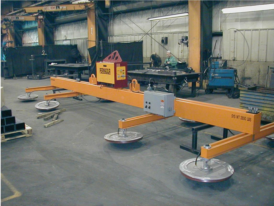
The above pictured System is a **PERMADUR Series 408 Plate/Part Handling System**. This System consisted of a 1500 Power Pac and eight Vacuum Pads on a 36' Load Beam. Eight VPN-24-30 Vacuum Pads on four Crossarms support 10'x40' Plate Loading. The System Load beam was designed to be attached to a Double Hook Crane. The System is powered by a 460 VAC power supply and provides an Interface with Crane Radio Remote ON/OFF/OFF Controls.
